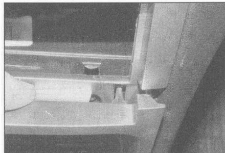
27.12 Starting at the top, prise the panel from place
