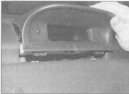
27.25 Pull up the rear of the unit to release the clips (arrowed)
