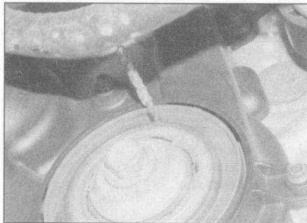
3.11 Insert a 5 mm drill through the hole in the crankshaft sprocket flange, and into the corresponding hole in the oil pump
