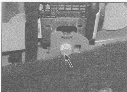
24.5a Undo the seat belt lower anchor bolt (arrowed)
