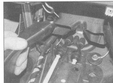
3.5 Remove the air ducts from above the gear lever housing
