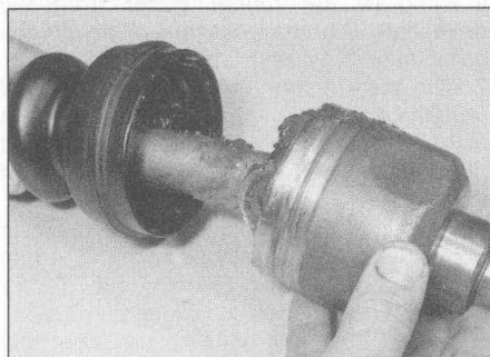
3.16a Release the inner gaiter retaining clips, and remove the joint outer member
