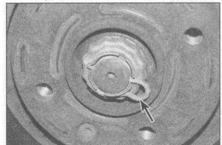
2.1 Prise out the R-clip (arrowed), remove the locking collar and slacken the driveshaft nut
