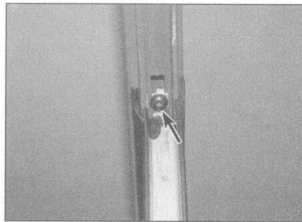
14.41 Undo the quarter light frame retaining screw (arrowed)
