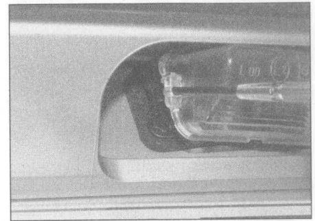
5.37 Prise the side of the lens out to release it from the clip
