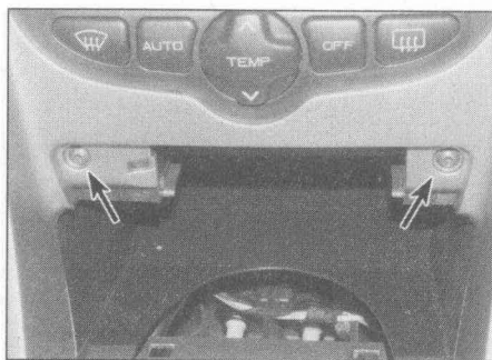
10.3 Undo the two screws (arrowed) below the control panel
