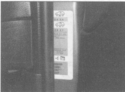
The vehicle production and paint codes are located on the driver's door pillar
