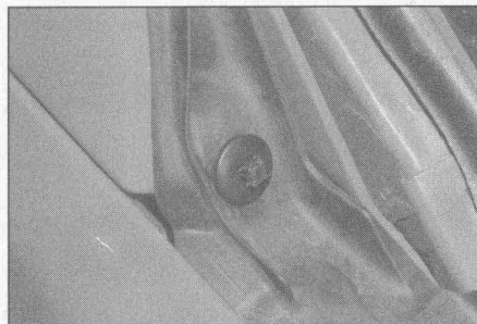
2.39a Push in the centre pins a little, then prise out the complete plastic expanding rivets . . .
