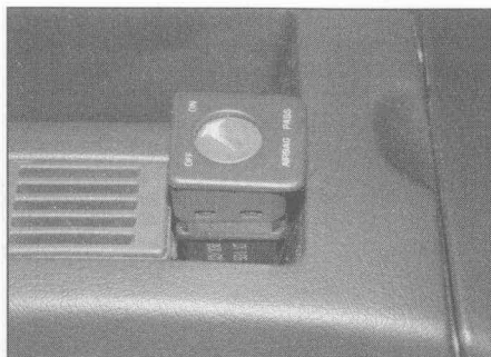
26.4 Prise up and disconnect the airbag disarming switch
