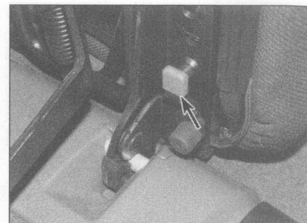
23.14 Release the clip (arrowed) and lift the seat from place
