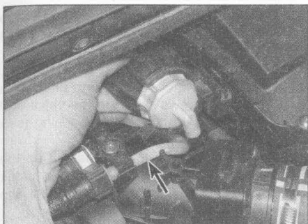
3.1 Operate the hand priming pump until fuel clear of bubbles appears in the fuel pipe (arrowed) (1.4 litre engine)
