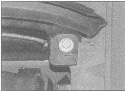
13.1d The plastic crossmember is secured by a bolt at each end
