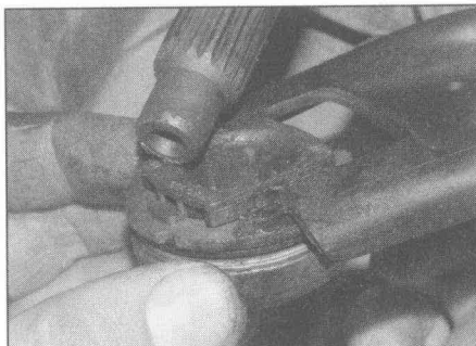
7.3 Disengage the release bearing from the release fork
