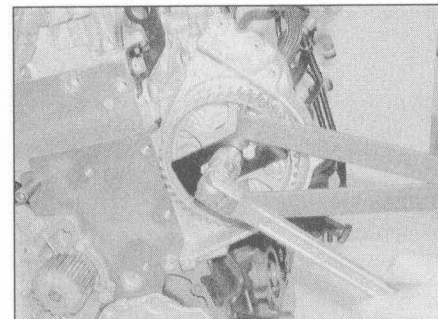
10.15 Using the home-made tools to remove the fuel pump sprocket
