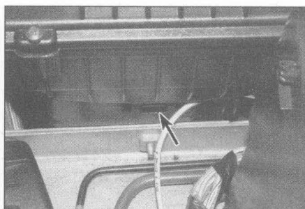
2.2 Depress the retaining clip (arrowed) and lift the air cleaner housing from its bracket
