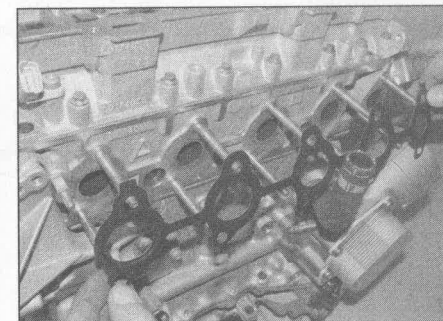
15.2b Recover the manifold gasket
