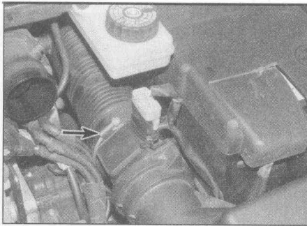
4.8 Slacken the clip (arrowed) and disconnect the flexible ducting from the air mass meter
