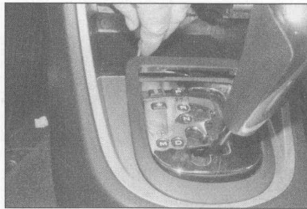
27.11b ... or prise up the selector lever position display trim on automatic transmission models
