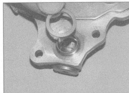
12.21a Fit a new oil seal . . .
