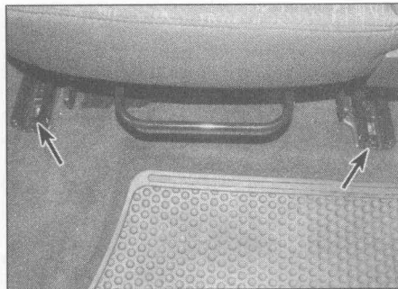
23.5 Undo the two bolts at the front of the seal rails (arrowed)
