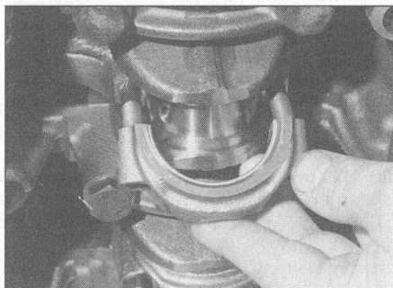
9.5 Remove the big-end bearing shell and cap
