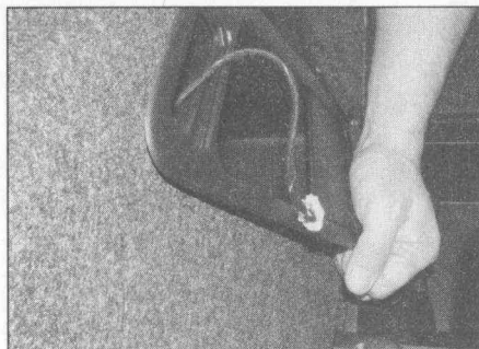
25.46 Remove the storage compartment trim surround
