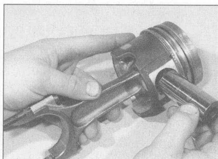
12.15b . . . and withdraw the gudgeon pin
