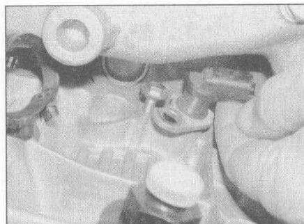
13.19 Turn the sensor body to clear the bolt and withdraw it from the bellhousing
