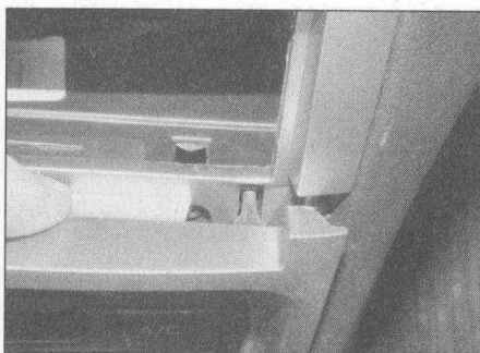
10.5 Starting at the top, unclip the trim panel
