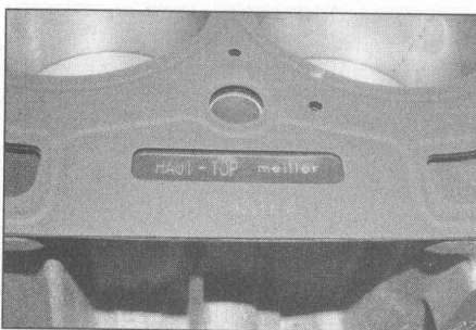
11.28 Position the cylinder head gasket with the work TOP uppermost and toward the oil filter side of the engine block
