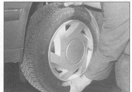
13.4 Check for wear in the hub bearings by grasping the wheel and trying to rock it
