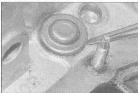
10.21 On 1.4 litre diesel engines, prise up the two caps to expose the main bearing bolts at the flywheel end
