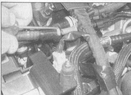
6.7 Disconnect the fuel supply and return hose quick-release fittings
