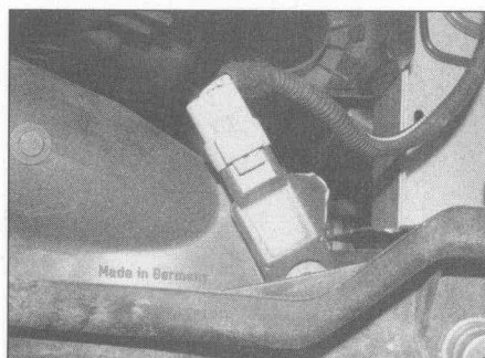
18.8 Disconnect the sensor wiring plug
