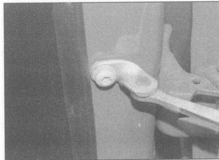
11.3 Undo the door check strap bolt
