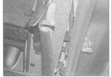
25.43 Unclip the lower C-pillar/rear door sill plastic trim
