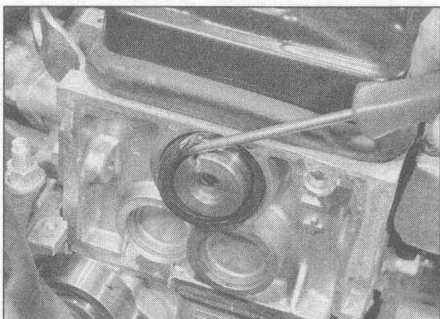
8.2 Carefully prise the camshaft oil seal out with a flat-bladed screwdriver
