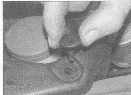
13.7 Push in the centre pin a little, then prise out the complete plastic expanding rivet
