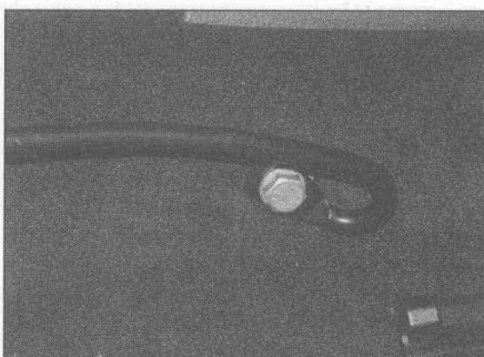
24.5b Prise off the rubber cap and undo the anchor bolt (3-door model)
