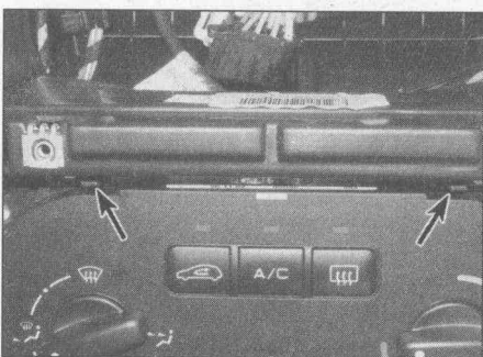
10.6b . . . and release the retaining clips (arrowed)
