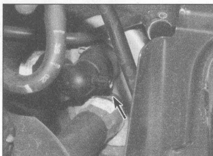
22.5 Undo the bleed screw from the heater outlet hose union (arrowed)
