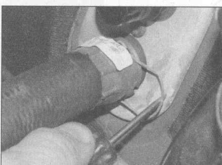
10.15 Prise out the wire retaining clip and disconnect the heater hose
