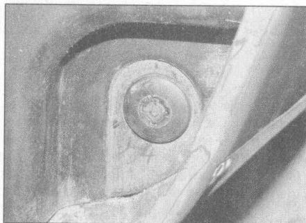
19.2 Push in the centre pin, then lever out the complete plastic rivet
