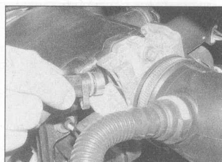
13.44 Remove the throttle housing heating element (1.4 litre engine)
