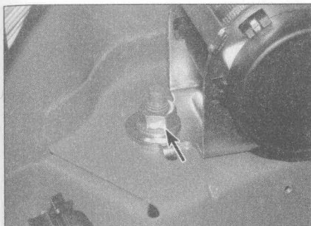
24.9 Undo the seat belt reel nut (arrowed)
