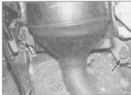
19.9 Catalytic converter mounting bolts (arrowed)
