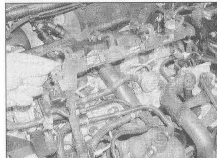
11.12 Undo the two nuts and lift off the plastic wiring harness guide
