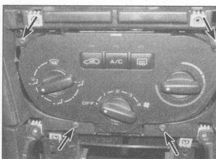
10.6a Undo the four heater control panel retaining screws (arrowed) . . .
