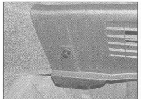
25.74 Remove the plastic rivet at each end of the tailgate sill trim (Hatchback models)
