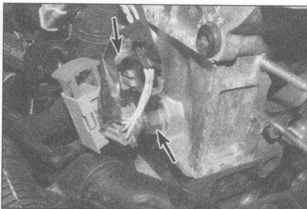
7.1a Coolant temperature sensors (arrowed) (1.6 litre petrol engine, 1.4 litre similar) ...
