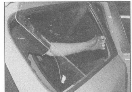
14.29 Lift up the rear end and manoeuvre the window from the door
