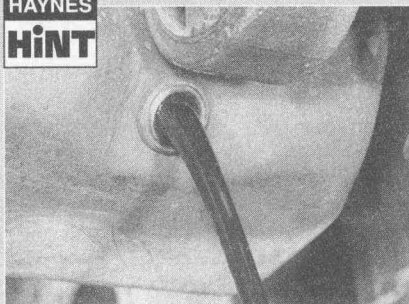
3.4 Slacken the sump drain plug
