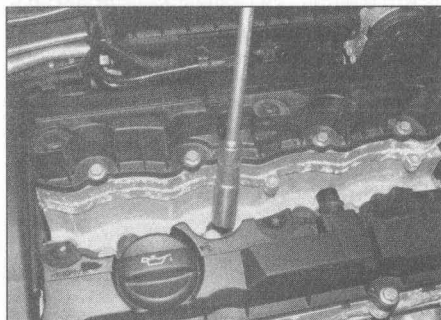
16.3 Unscrew the spark plugs
