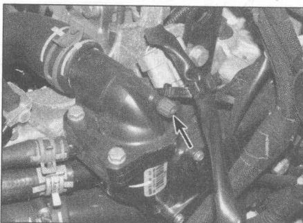
21.9a Coolant outlet housing bleed screw (arrowed) ...
