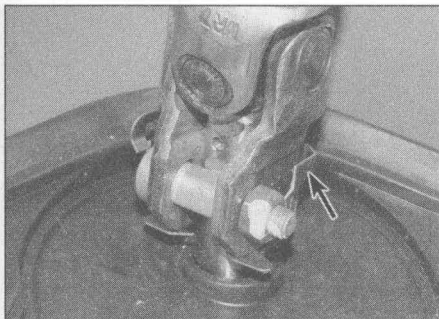
18.3 Release the retaining clip (arrowed) then remove the pinch-bolt/nut
