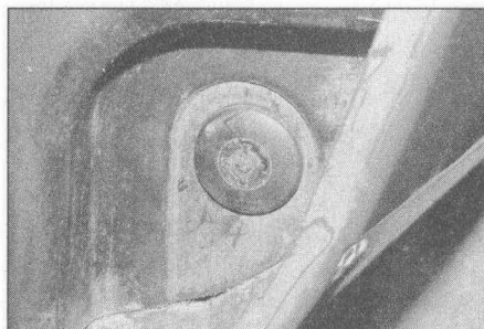
10.6a Push in the centre pins a little, then prise out the complete plastic expanding rivets . . .
