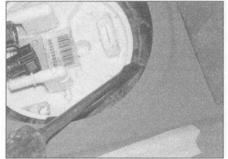
8.5 Tap the screwdriver to rotate the locking ring anti-clockwise
