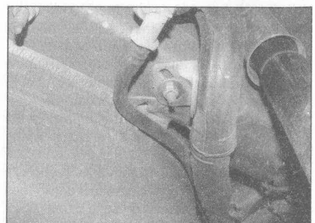
10.11e ... and lower fixing bolts
