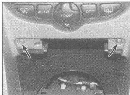
27.9 Undo the two screws (arrowed) above the ashtray aperture
