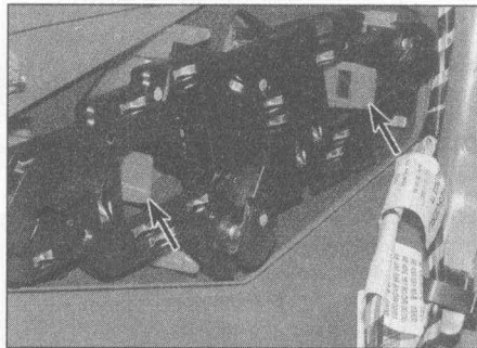
5.29 Squeeze together the tabs (arrowed) and remove the bulbholder assembly
