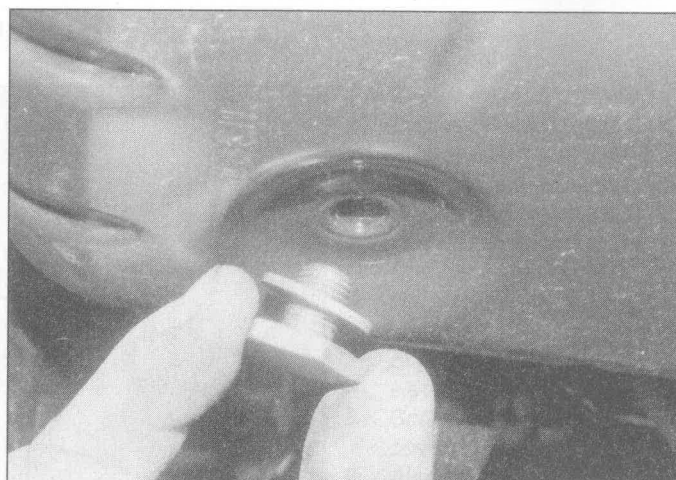
3.3 Unscrew the sump plug
