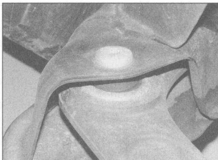
6.3 Undo the lower arm front pivot bolt ...
