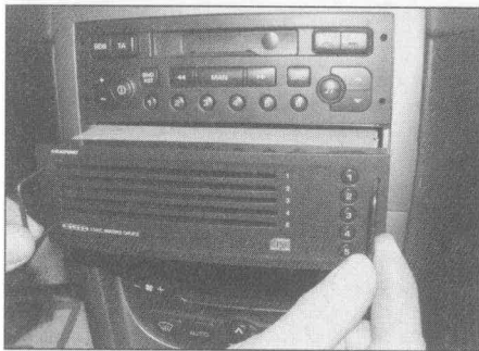
17.2 Insert two pins into each side of the audio unit to release the clips, then pull the unit from place
