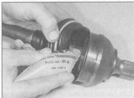
3.11f Pack the joint with grease, working it into the ball tracks while twisting the joint, then locate the gaiter outer lip in its groove on the outer member
