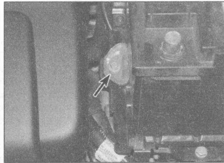
4.5 Undo the battery clamp bolt (arrowed)
