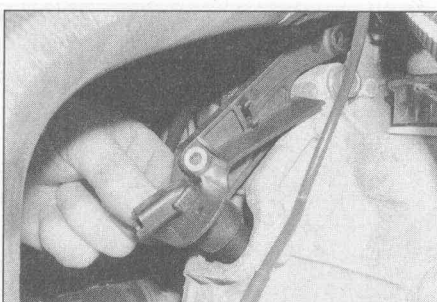
13.41b ... then remove the crankshaft position sensor from the front of the transmission housing
