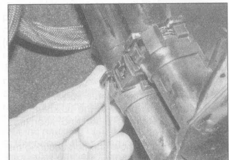
10.18c ... then release the retaining clips
