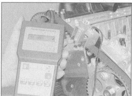
7.41b ... when the specified tension value is shown on the measuring equipment
