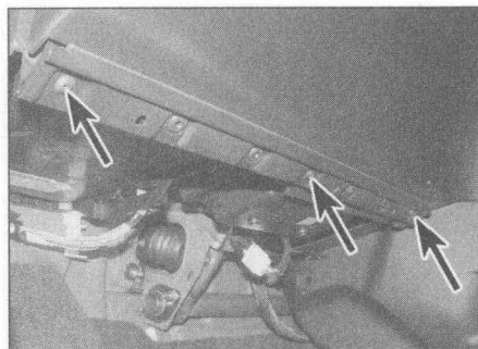
27.21b . . . and the 3 lower screws (arrowed)
